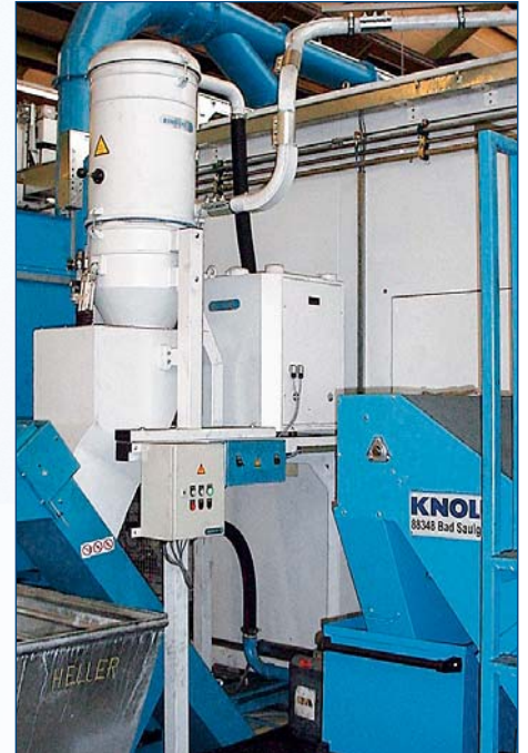
RA 240 D5.5 as chip extraction system with 1 to 2 suction points
