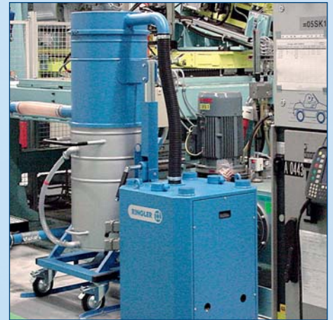
Drilling chips extraction in the automotive industry
