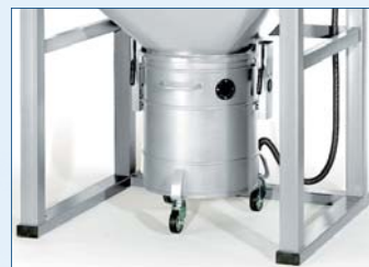
100l run-out collection tank
