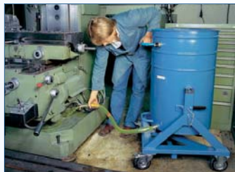
Level indicator hose to drain the coolant
