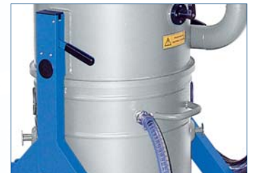
Lowerable steel collection tank 100l, mobile, handle, pressure compensating hose, PE round bottom bag with holding-down device for dust-free emptying
