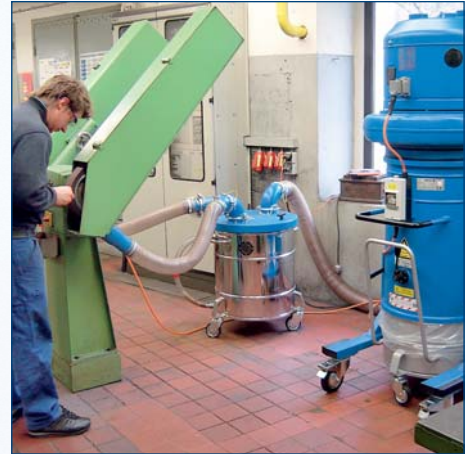
RI 334 with stainless steel pre-separator for the safe separation of dusts with flying sparks on 2 belt grinders.
