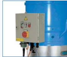
Control cabinet for motor, shaker and level sensor
