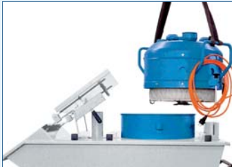
Raise the drive head by hand or crane
