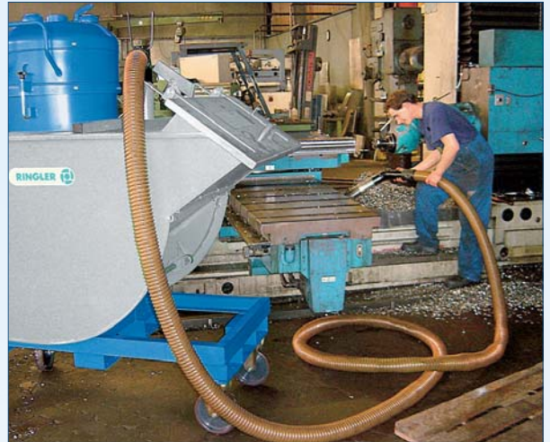
Suction extraction of large amounts of chips and coolants
