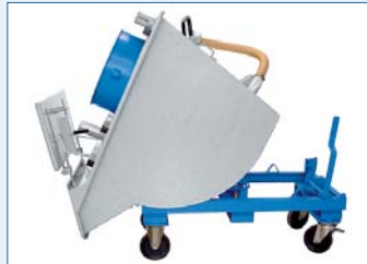
Emptying by tipping with integrated tip damper
